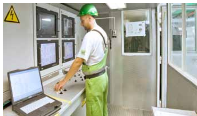
Operation of TBM
